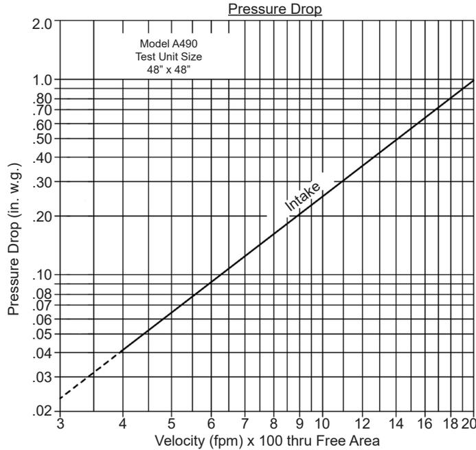
Intake air converted to standard air density.
